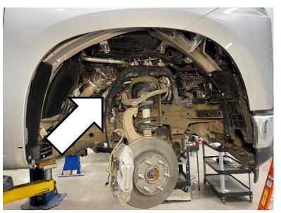
Remove the passenger side wheel, fender liner, and skid plates to get closer to the sensor. The sensor is behind a heat shield near the exhaust that can be unscrewed and moved out of the way as shown:
